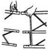
1.) Check the Instructions for your particular base to dig a proper size hole. Place each ten-foot tower section end to end in the correct order of assembly; start by putting the bottom section at which place the tower will stand. Make sure enough clearance exists so that the tower can later be walked up to its upright position without overhead interference.
